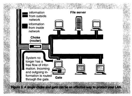
configuration, but they also add to the delay and difficulty involved with authorized network communication. For simplicity, the following sections assume that there is a single choke and a single gate, as shown in Figure 3.
