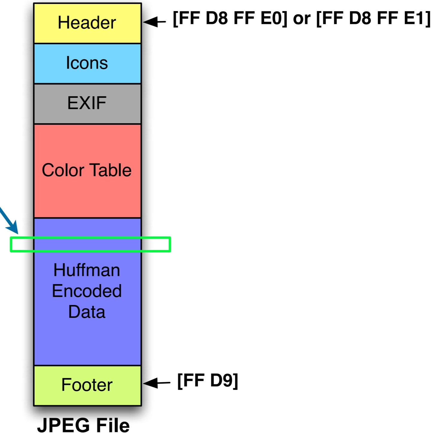
We built detectors to recognize the different parts of a JPEG file.
