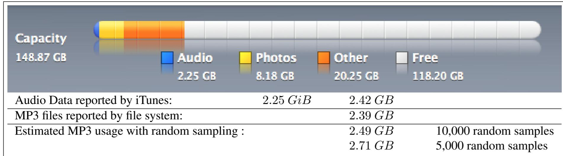
**Figure 1:** Usage of a 160GB iPod reported by iTunes 8.2.1 (6) (top), as reported by the file system (bottom center), and as computing with random sampling (bottom right). Note that iTunes usage actually in GiB, even though the program displays the “GB” label.
