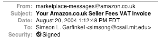
Figure 2. Apple’s OS X Mail application displays a special “Security:” header to indicate if messages are digitally signed.
