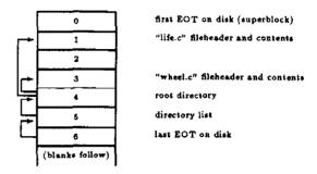
Figure 1: Direct Read After Write disk after a sample transaction
