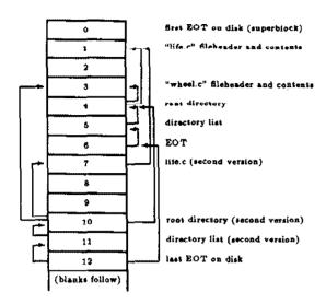
Figure 2: Direct Read After Write disk after a second sample transaction. Arrows on the left hand side trace pointers from the EOT to the most current version of each file. Arrows on the right hand side trace pointers to previous versions.
